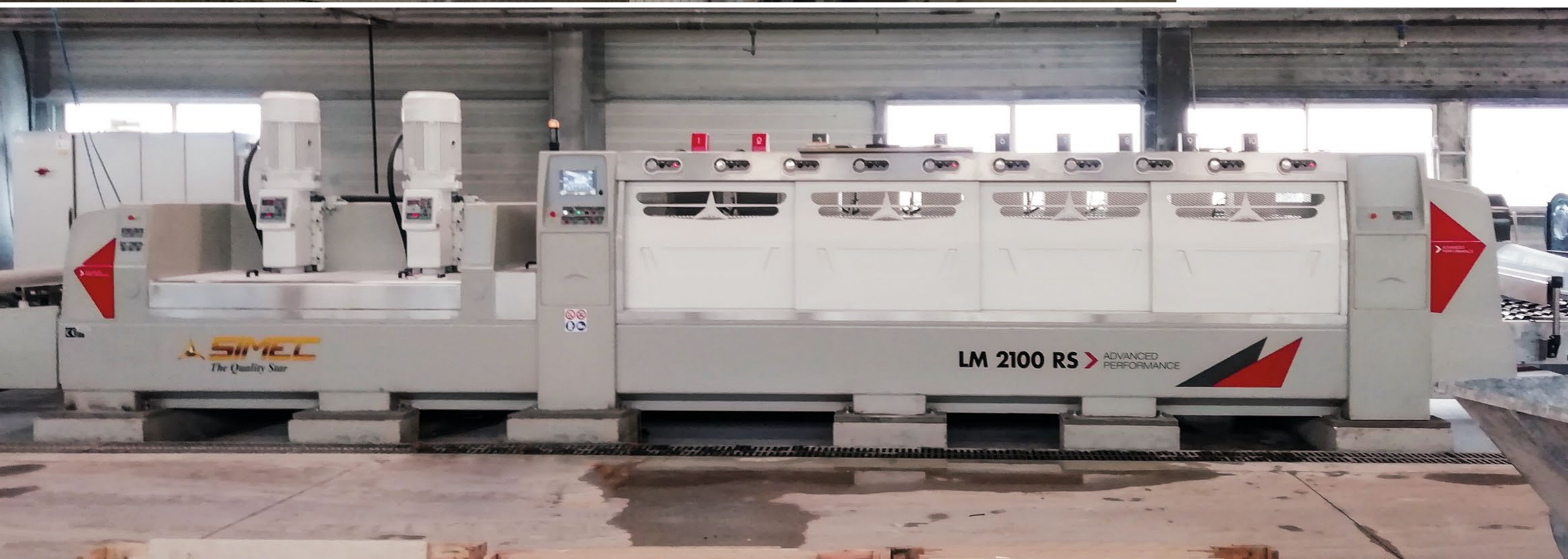
Below: combined calibrating-polishing machine for marble slabs model LM 2100 RS 210
